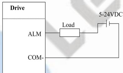
**Figure 5** Sinking output
