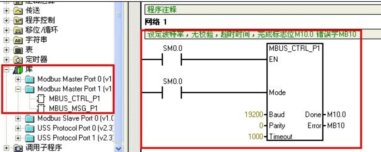
Figure 9-11 S7-200 PLC communication parameters
