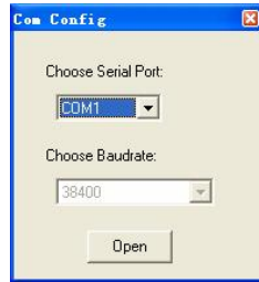
Figure 21: RS232 communication configuration window
