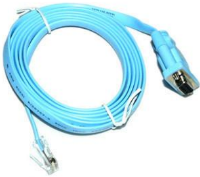
Figure 9-1 Serial port to RJ45 line
