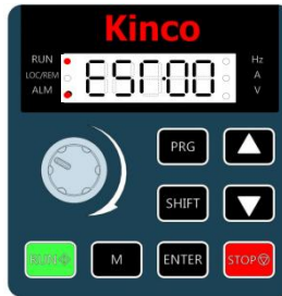
Figure 5-29 Self learning mode operation panel
