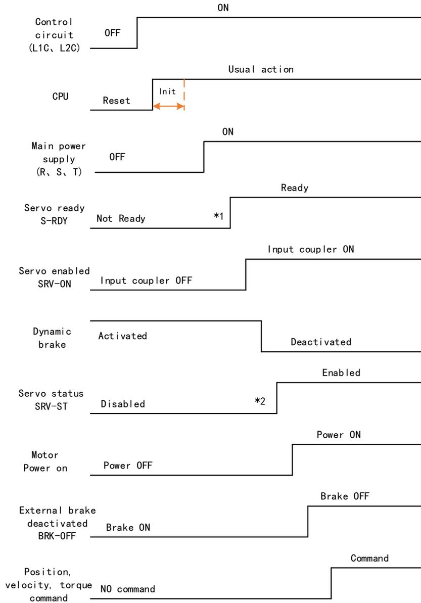
Please enter servo status, position, velocity, torque command as sequence diagram above.
