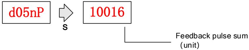
Press ◀ to switch between high/low bit
