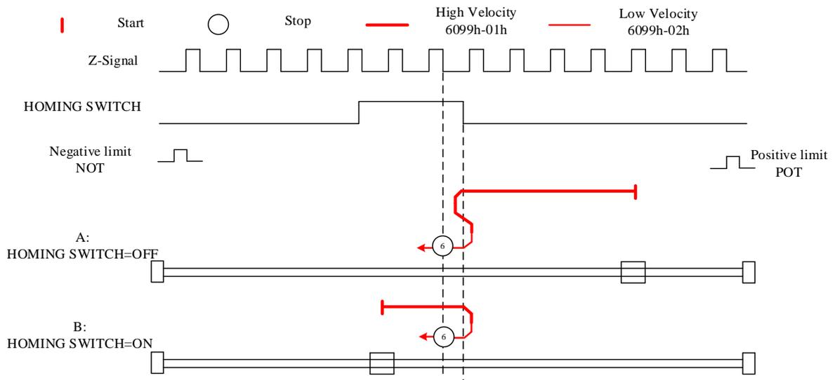
**Limit switch signal + homing switch signal + Z-signal mode**
