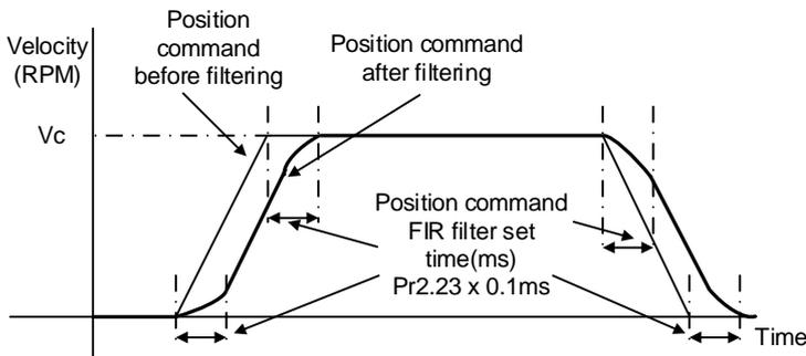
Usually applied when there is rather sharp acceleration which might cause motor overshoot or undershoot. To smoothen command signal, reduces impact to machines and eliminate vibration. If Pr2.23 is set too high, overall time will be lengthened.
