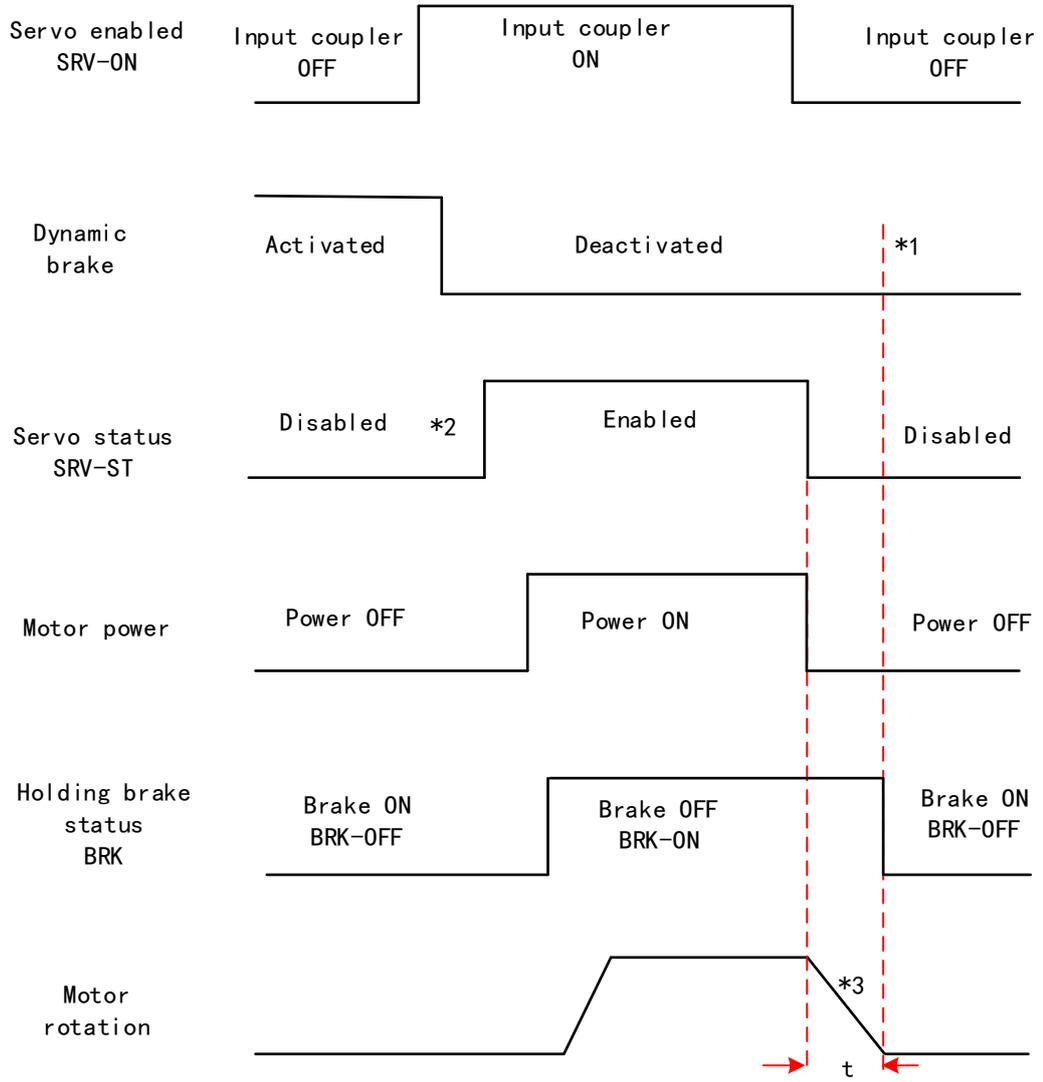
**Dynamic braking method. Status after stopping: Free moving**
