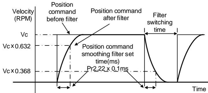
Usually applied when there is rather sharp acceleration which might cause motor overshoot or undershoot. To smoothen command signal, reduces impact to machines and eliminate vibration. If Pr2.22 is set too high, overall time will be lengthened.
