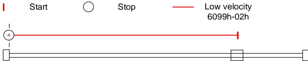
**Mode -5:** Search for homing point in **positive direction** at **low velocity**. Stop after torque reaches the value set in Pr5.39 and homing done signal delivers after the time value set in Pr5.37
