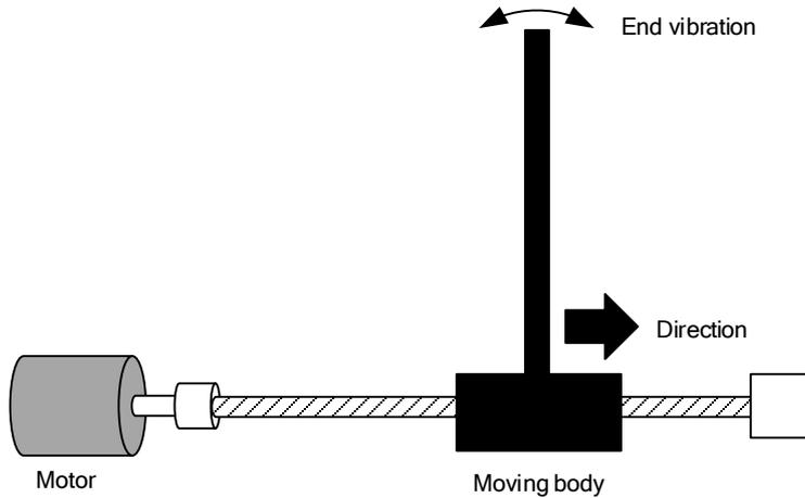
If the mechanical structure has an end that is long and heavy, it might cause end vibration at emergency stop and affect the positioning. Usually happens on long armed axis with loose end. The frequency is usually within 100Hz which is lower than mechanical resonant frequencies. It is called low-frequency resonance which can be prevented by applying low frequency suppression function.
