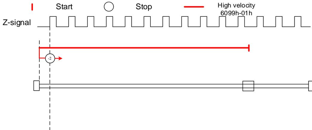
**Mode -1:** Search for homing point in **positive direction** at **high velocity**. Move in **negative direction** after torque reaches the value set in Pr5.39, stops when torque is gone with the **first Z-signal**.
