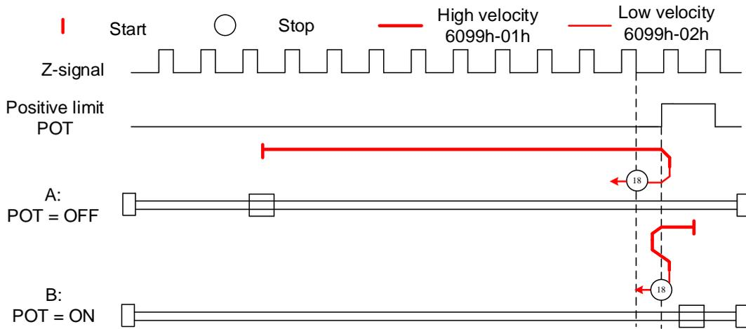
**Homing switch signal triggering detection mode**
