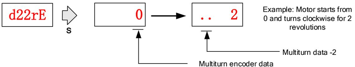
Multiturn encoder data range: -32768~+32767, As no. of revolution goes over range, 32767 will jump to -32768, -32767(counter clockwise); -32768 will jump to 32767, 32766 (clockwise)
