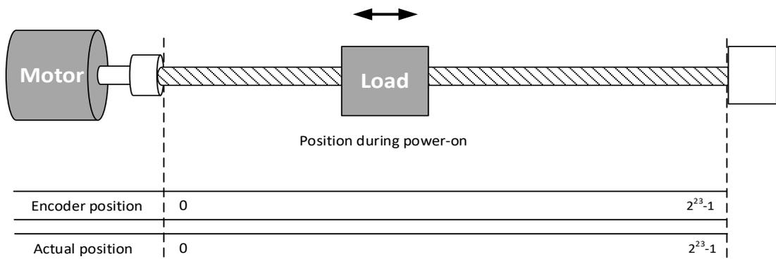
When electronic gear ratio = 1:1, 607Ch = 10000:
