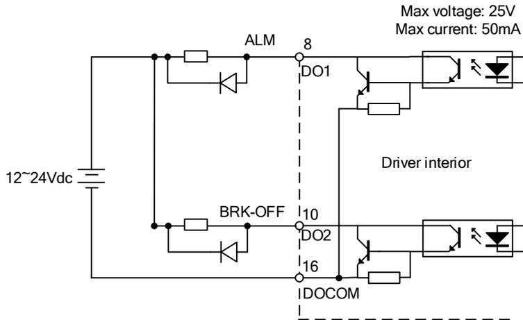
Please install flyback diodes (as shown in diagram above) if the output is through a relay or other inductive load to prevent damage to DO ports.
