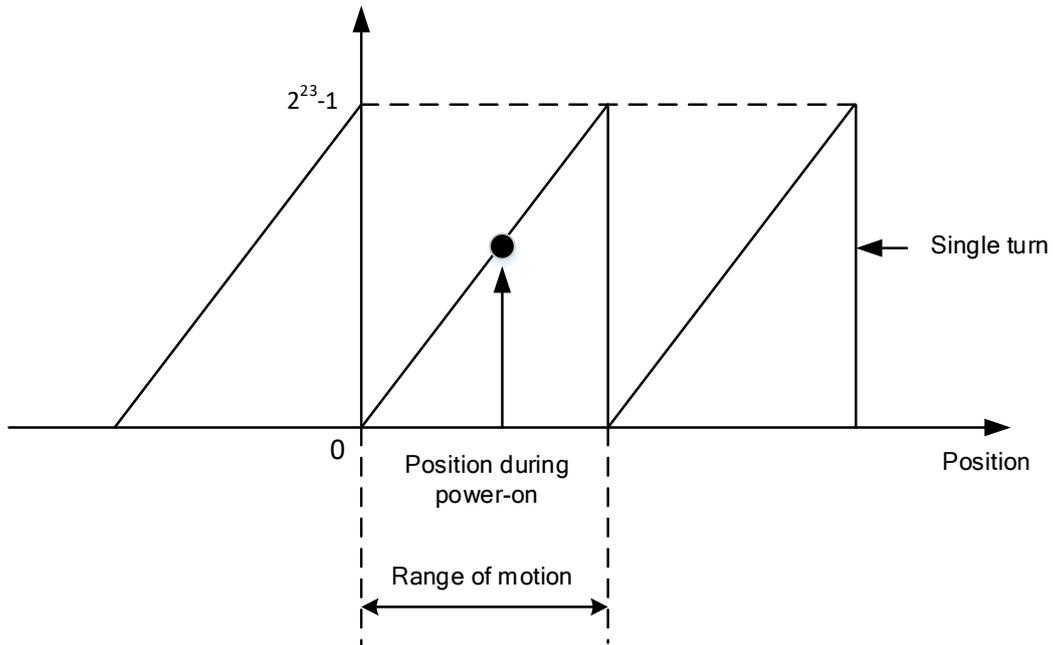
If power is turned off at position as shown below and power on when motor reaches the position below. Motor range of motion changes as shown below.
