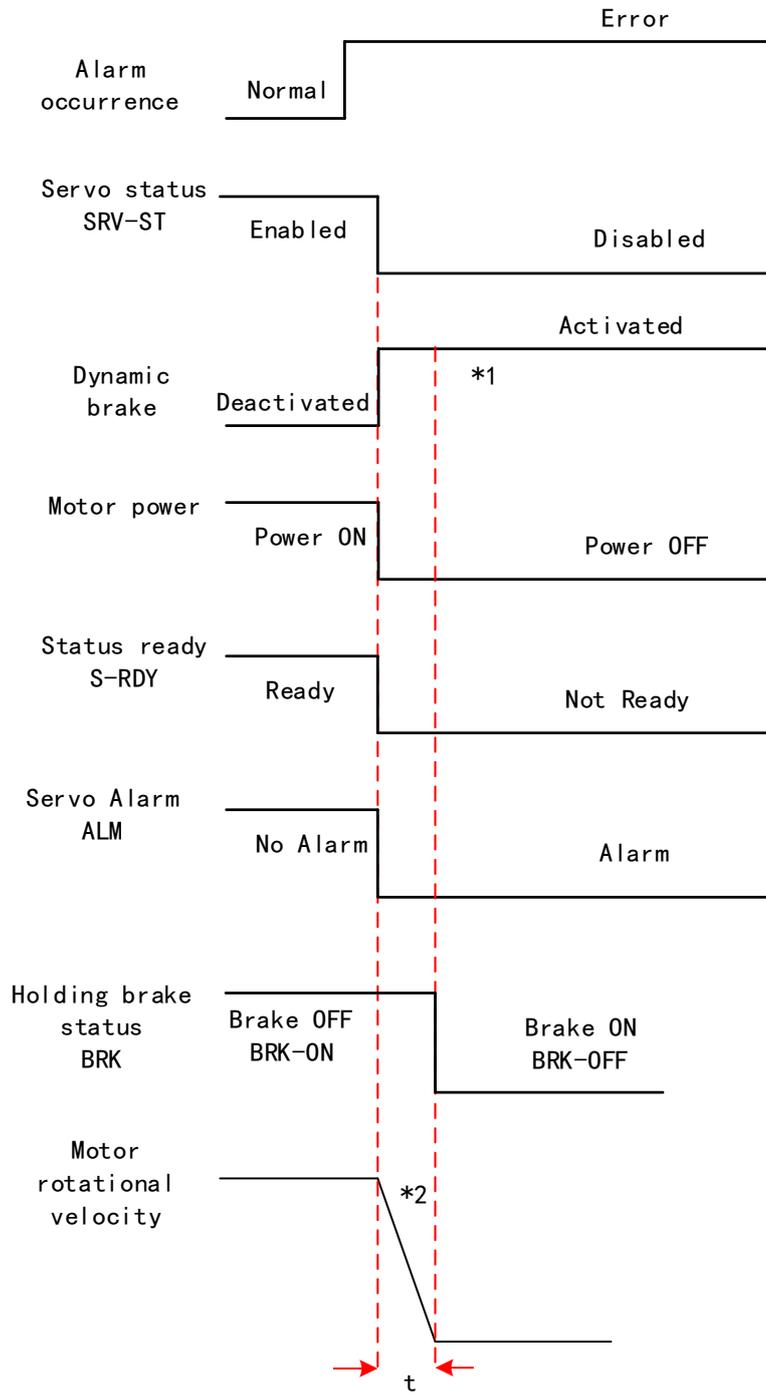
Servo braking method. Status after stopping: Free moving
