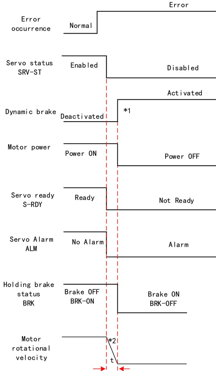
Free stopping method. Status after stopping: Dynamic braking
