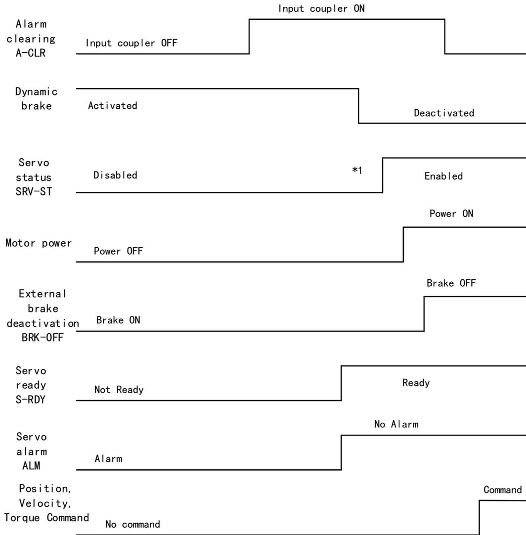
**\*\* 1.** SRV-ST signal is received when servo driver is enabled. Command input is not allowed yet
