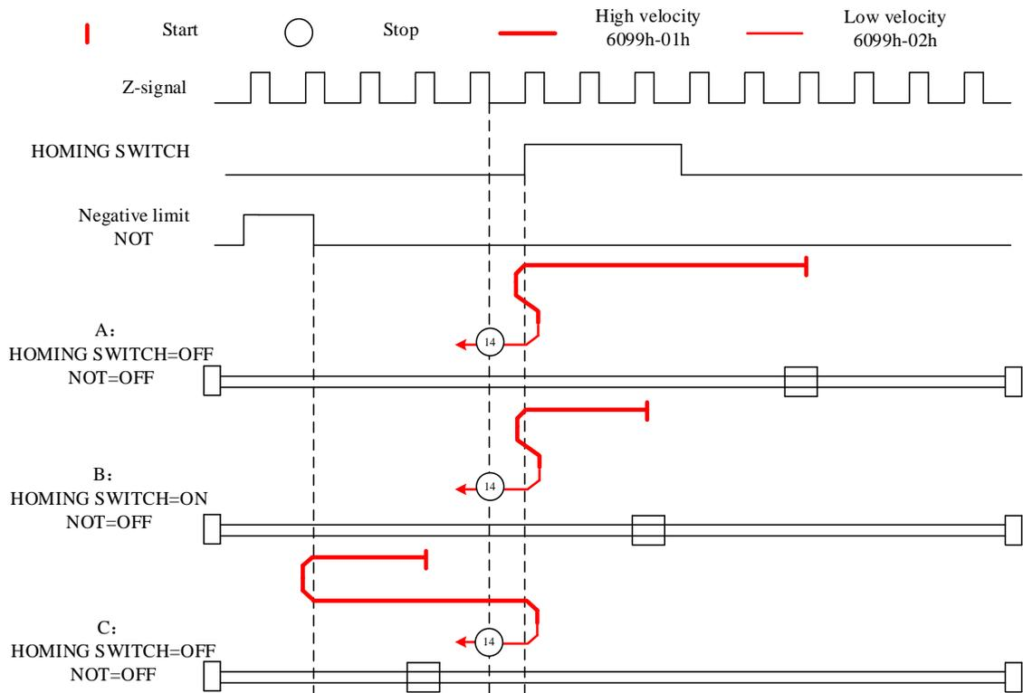
**Limit switch signal triggering detection mode**
