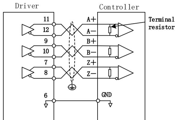
If controller input circuit is not an optocoupler input circuit but a differential receiving circuit, please connect CN5 pin 6 (OC reference ground) to GND of controller differential receiving circuit.
