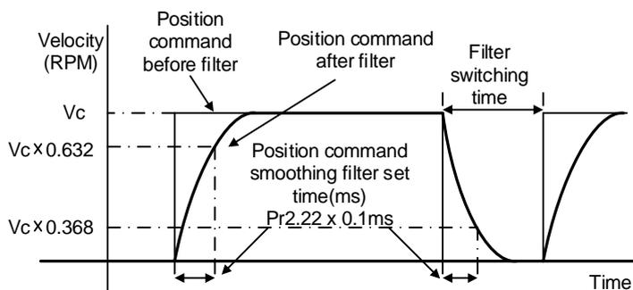
Usually applied when there is rather sharp acceleration which might cause motor overshoot or undershoot. To smoothen command signal, reduces impact to machines and eliminate vibration.
