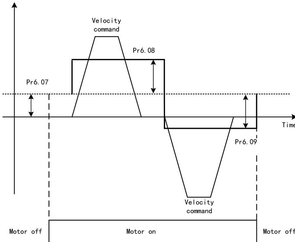
Vertically loaded axis: A constant eccentric load torque is applied on the motor. By adjusting Pr6.07, positioning deviation due to different motional direction can be reduced.
