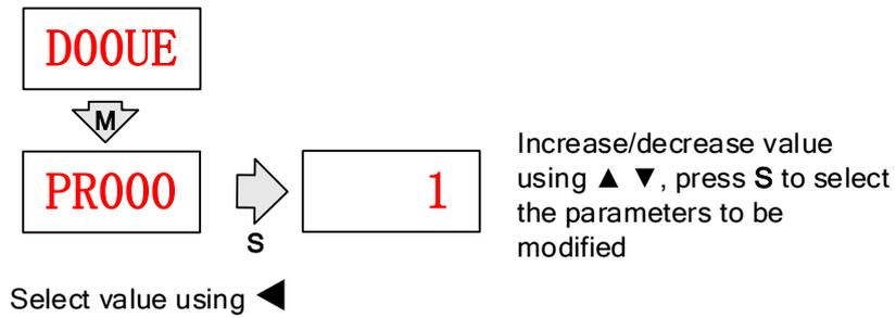
After modifying the selected parameter to desired values, press **S** to confirm and save the changes.
