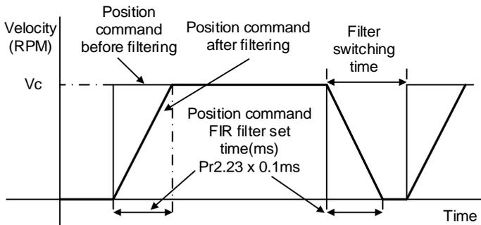
As shown below, when target velocity  $V_c$  trapezoidal command reaches  $V_c$ , it becomes S wave after filtering.
