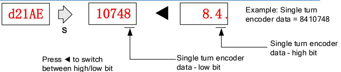
For 23-bit encoder, single turn encoder data = 0~8388607. Each value corresponds to certain position in a single revolution of the rotor, clockwise motion as negative, counter clockwise motion as positive. When counter clockwise single turn data > 8388607, multiturn data +1, clockwise single turn data < 0, multiturn data -1.
