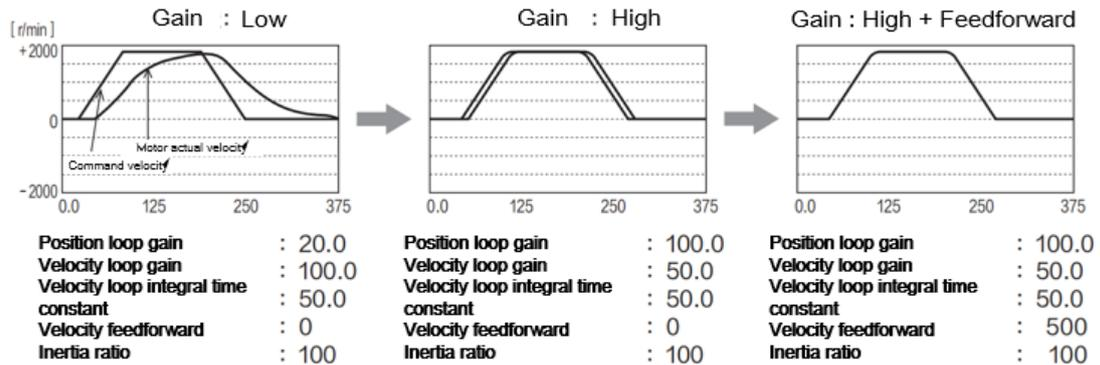
Servo driver gain adjustment is done in combination with a few other parameters (Inertia ratio, Position loop gain, Velocity loop gain and Filters settings). These parameters will have an effect on each other so it is always advisable to tune each parameter according in order to achieve optimal machine performance. Please refer to the steps below
