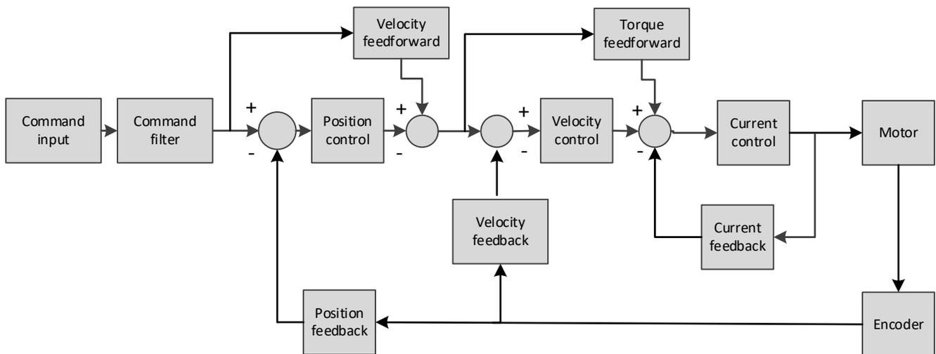
Inner control loop demands higher responsiveness. In order to avoid system instability, please tune in accordance to this principle. Current loop gain usually satisfies the responsiveness demand without tuning. When gain adjustment is done under position control mode, in order to keep the system stable, position and velocity loop gain have to be increased at the same time to make sure the responsiveness of the position loop is lower than velocity loop.
