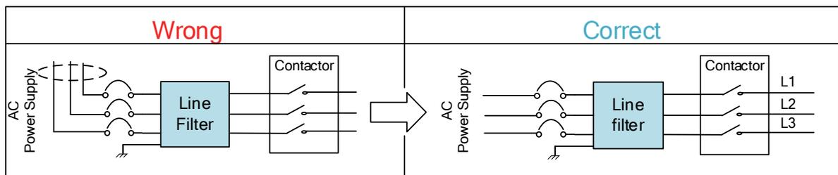
Separate the ground wire from the line filter and the main power supply cable.
