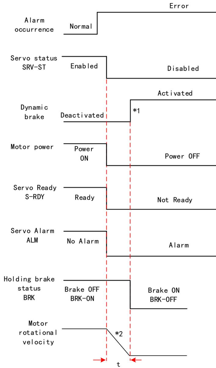
Dynamic braking method. Status after stopping: Dynamic braking
