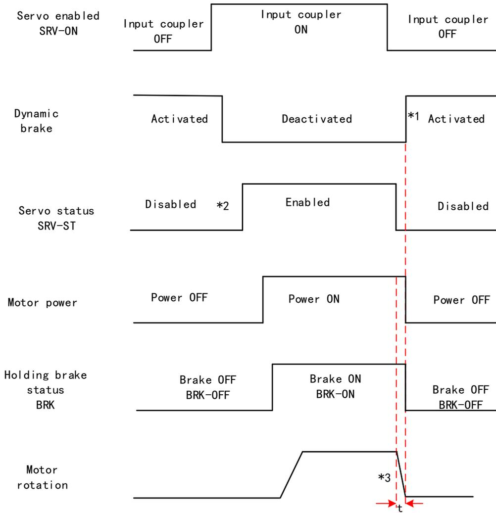
Servo stopping method. Status after stopping: free moving
