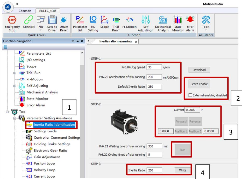
5. After the calculation is done, inertia ratio will be calculated automatically and click on 'write' to enter the calculated value into Pr0.04.
