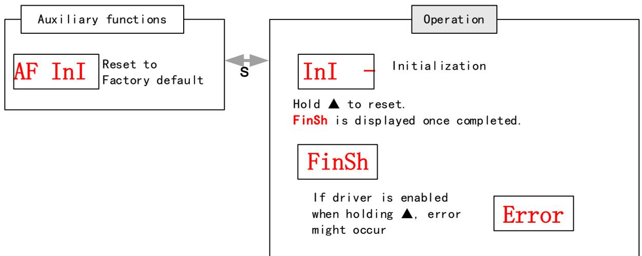
**Reset to factory default using object dictionary**
