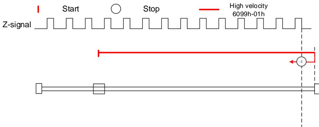
**Limit switch signal + Z-signal mode**
