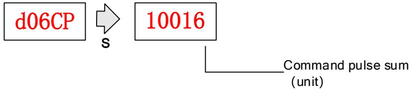
Press ◀ to switch between high/low bit
