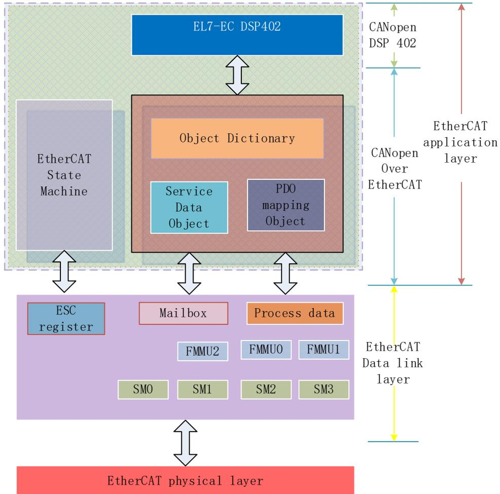
**Figure 7.4 The structure of EL7-EC network module**
