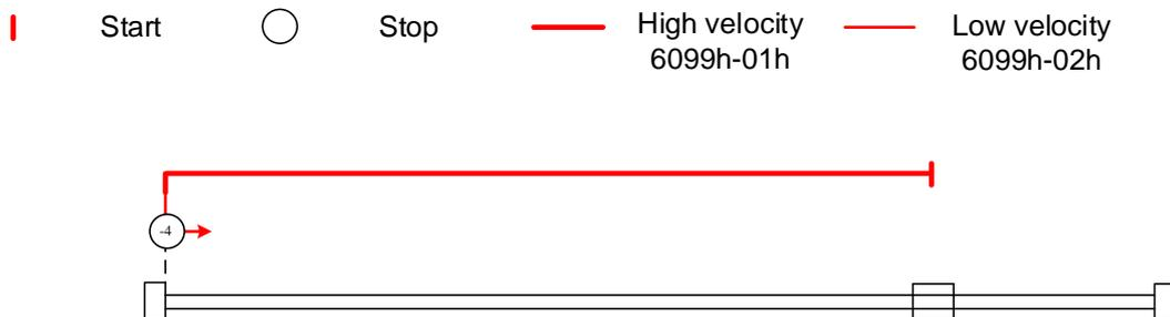
**Mode -3:** Search for homing point in **positive direction** at **high velocity**. Move in **negative direction** after torque reaches the value set in Pr5.39, stops when torque is gone. Homing done signal delivers after the time value set in Pr5.37
