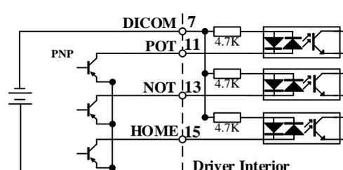
*Please prepare switching power supply with output of 12-24VDC, current  $\geq 100\text{mA}$ ;*
