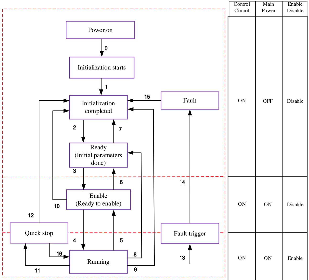
Figure 5.1 EL7-EC 402 State Machine switchover diagram
