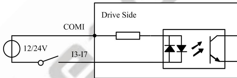
COMI: can be connected to 12 / 24 V (common-anode), or 0 V (common-cath)
